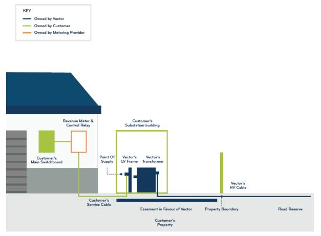
Option 2: Vector installs its own substation (transformer and LV frame in an outdoor enclosure) inside the customer's property.
