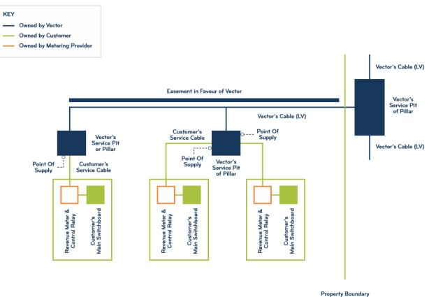
Note: Vector accepts reticulating inside right of ways provided that the customer agrees to grant an easement in favour of Vector (where required) to protect the equipment and allow Vector to operate and maintain the equipment. Vector will keep / maintain records of this equipment and the easement protecting it.
