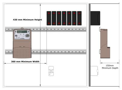
• Single phase installation – 430mm Height x 360mm Width x 150mm Depth
