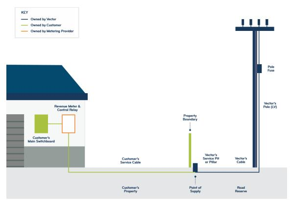
The diagram above shows a typical single dwelling that is connected to Vector's electricity network. For this type of connection, the customer owns and is responsible for the electrical equipment inside their property up to the Point of Supply.
